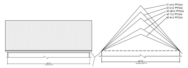
\*note: this roof has a 12 inch overhang (horizontal distance from siding to roof edge) on the front, back, and sides.
